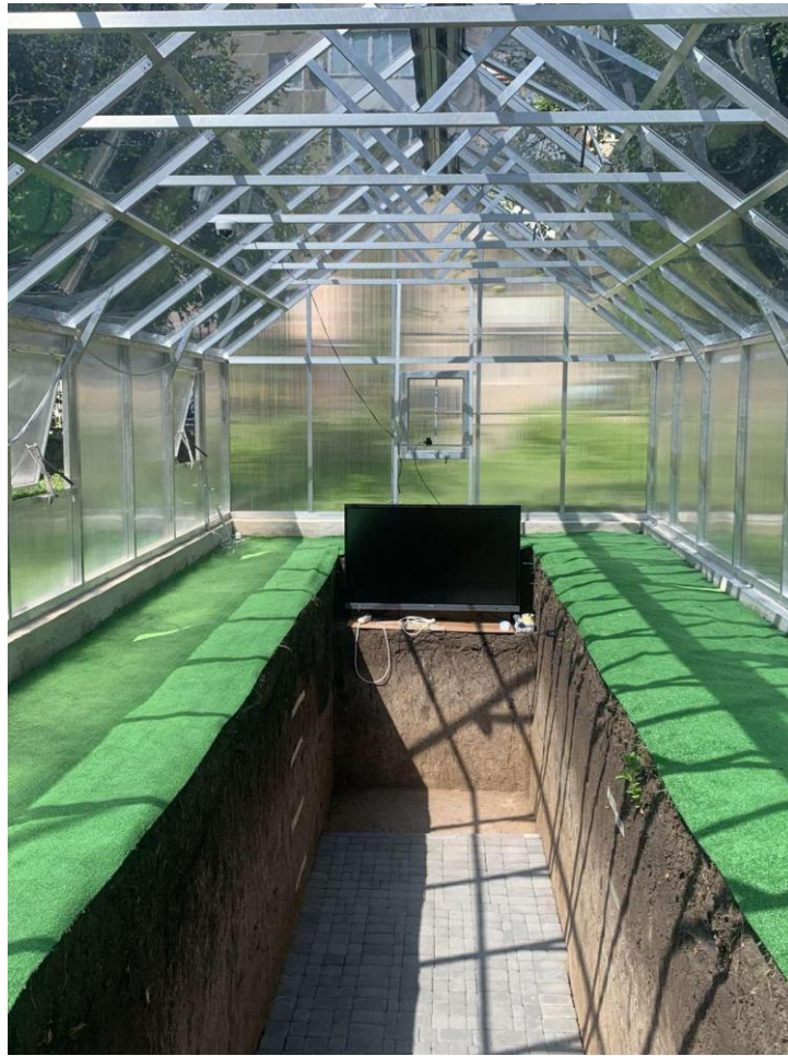
Figure 6. The opposite-to-stairs wall equipped with a sensor panel for monitoring
