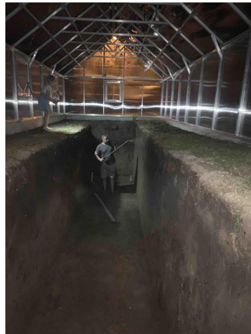
Figure 10. Structural stabilization of the exposed profile wall using a double application of PVA solution
